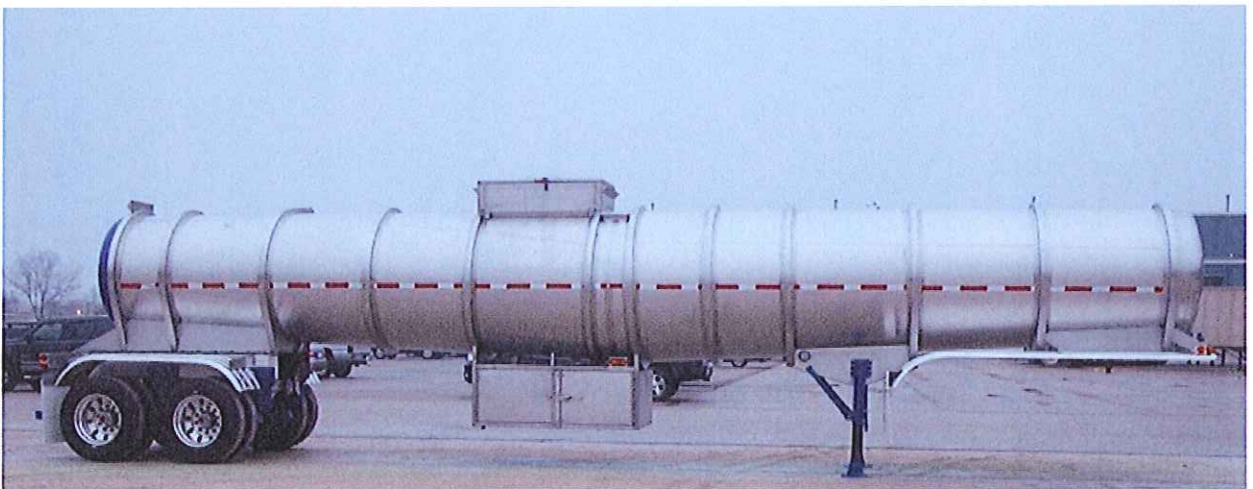
Figure 6: A Cargo Tank Motor Vehicle without any Ladder or Walkway
