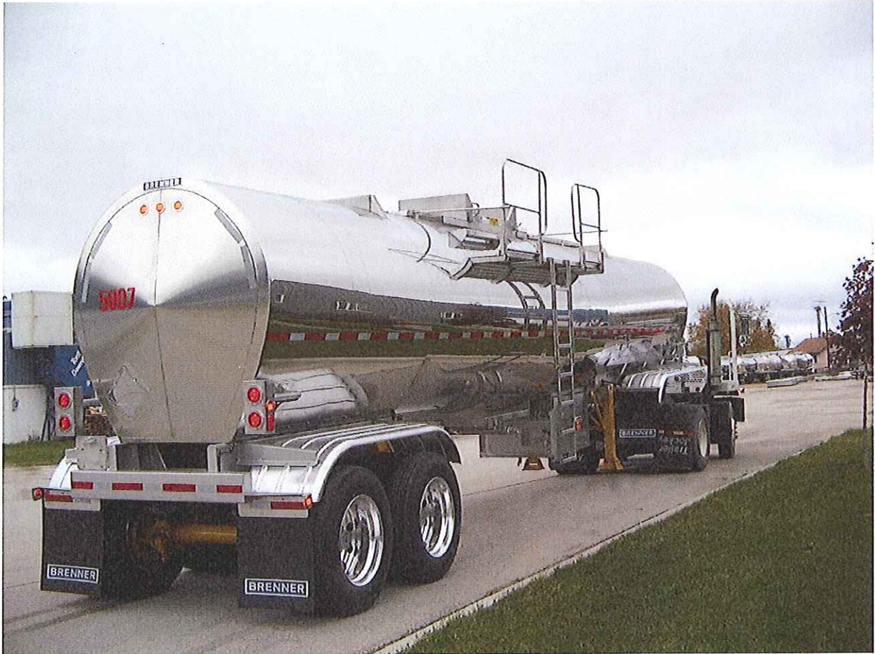
Figure 3: A Cargo Tank Motor Vehicle with a “Balcony Ladder” System and Additional Side Hand Rails
