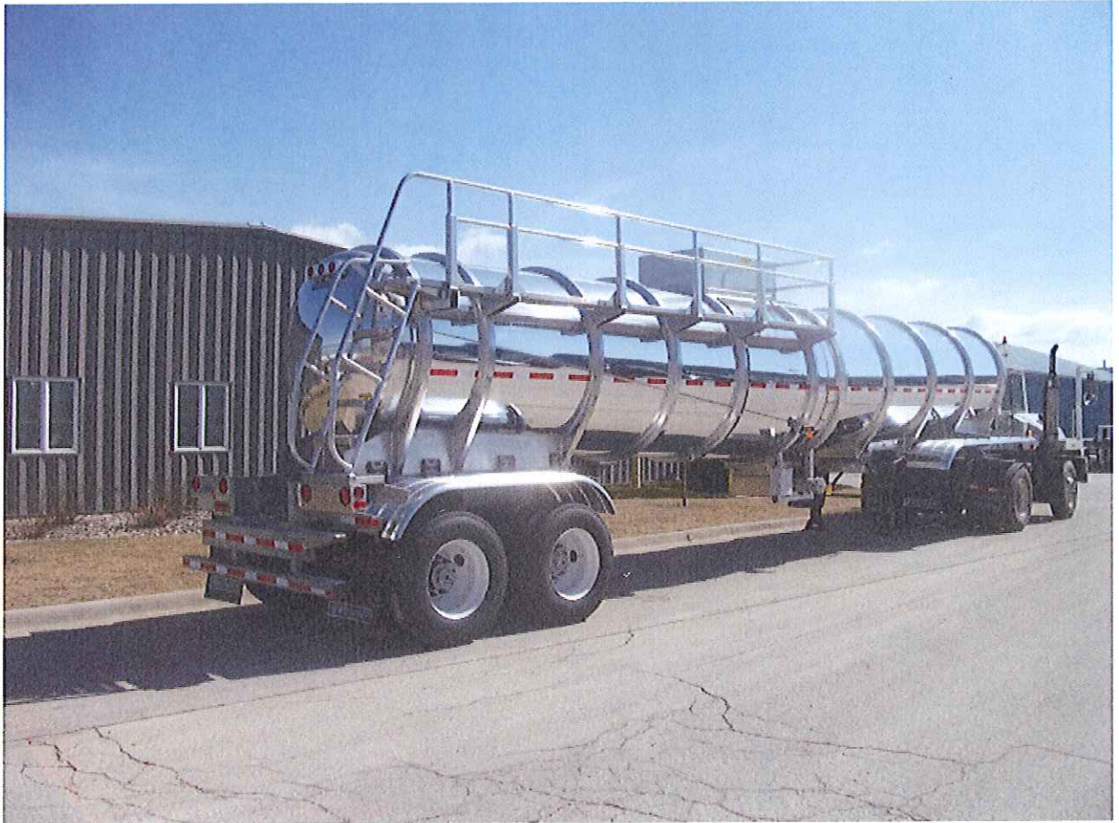
Figure 4: A Cargo Tank Motor Vehicle with an Angled Rear Access Walkway System
