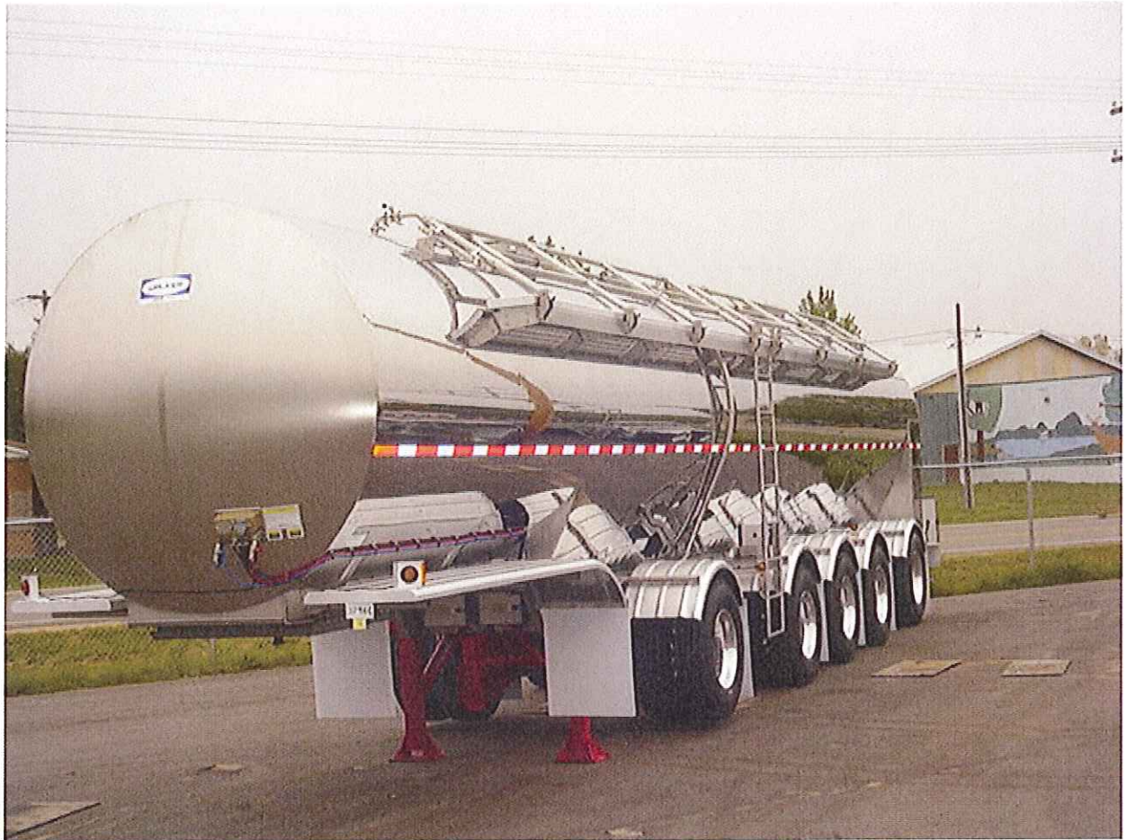
Figure 2: A Cargo Tank Motor Vehicle with a Collapsible Outer Railing
