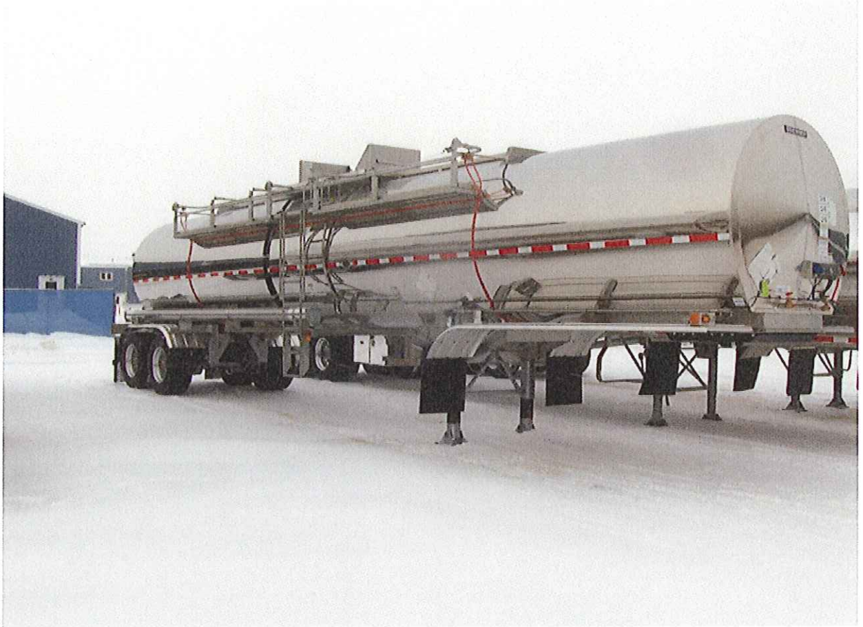
Figure 5: A Cargo Tank Motor Vehicle with a Pneumatically Actuated Outer Hand Rail
